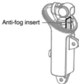
2. Power off Osmo Pocket, place it in the waterproof case as shown, and attach the anti-fog insert (included).
